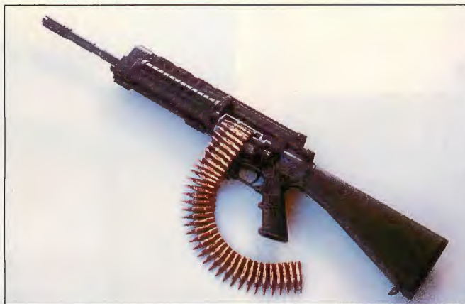
Johnston tested a special version of the Rigid Frame System with a belt-feed mechanism.
