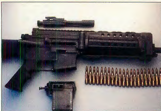
The Colt M16 belt-feed is seen here with its major components removed. Note the operating-cam groove in the bolt carrier.
