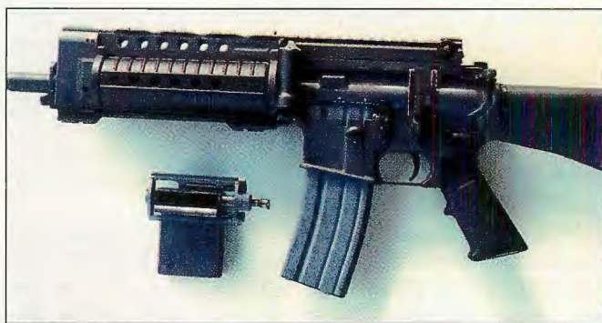
The Colt M16 belt-feed can be quickly converted to use a standard M16 magazine as seen here.
