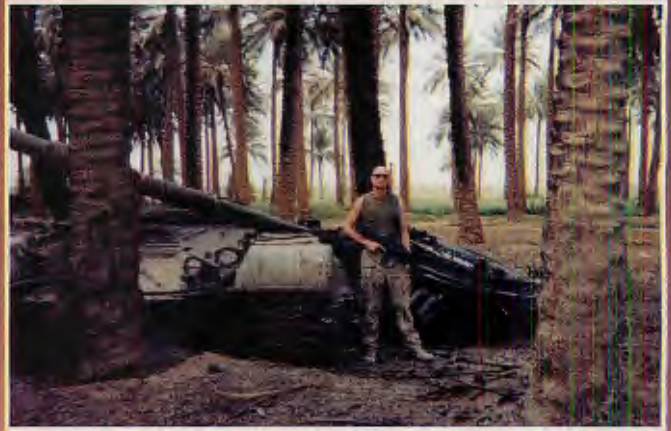
(above) T-72 killed by 25mm fire from Bradley, and (above, right) shows typical catastrophic hull failure, turret separation.
